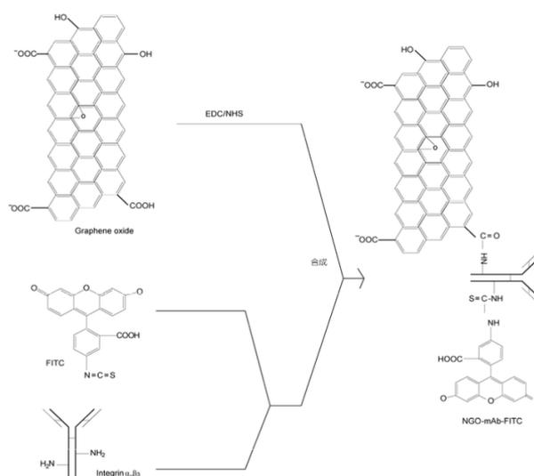
Figure 1. Flow chart of nanoprobe NGO-mAb-FITC construction
